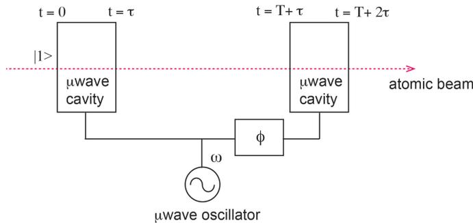
Figure 1: Ramsey spectroscopy setup.
