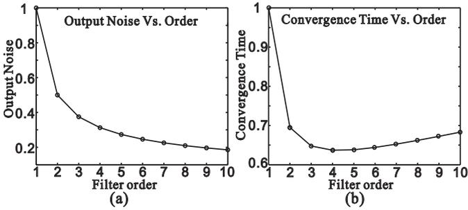
Fig. 4. (a) LPF output noise (normalized to the 1st-order value) vs. LPF order. The LPF's bandwidth is fixed. (b) Convergence time (normalized to the 1st-order value) vs. LPF order. Total LPF output noise energy is fixed.
