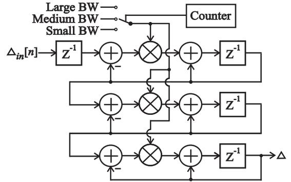
Fig. 5. 3rd-order discrete-time IIR LPF with a variable bandwidth scheme.
