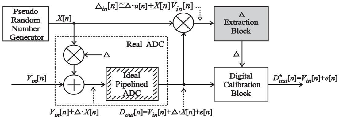
Fig. 1. Correlation-based digital background calibration.
