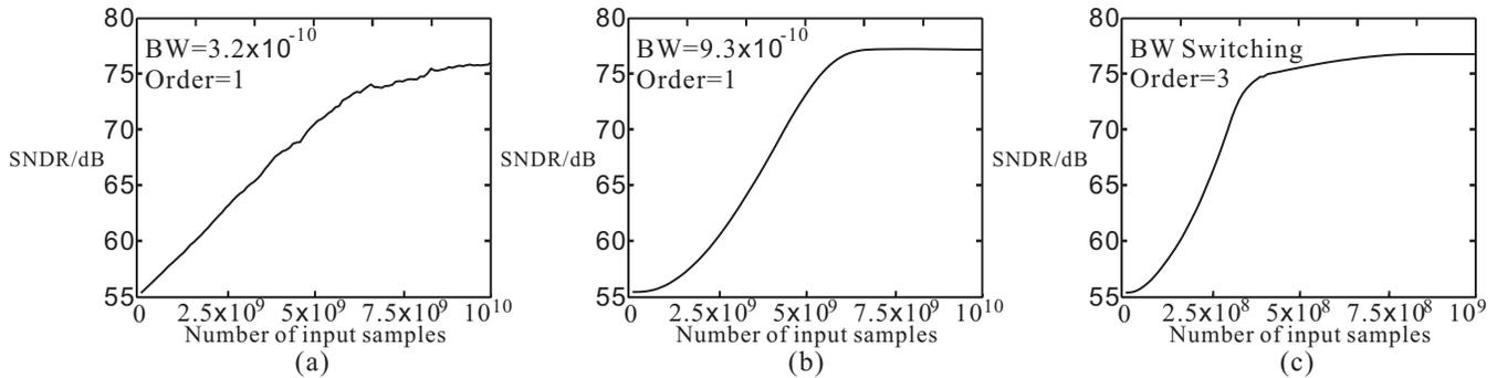
Fig. 6. Simulated convergence transients for a 13-bit pipelined ADC, for varying LPF bandwidths and orders.
